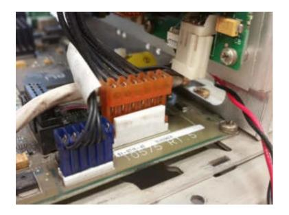
Remove blue connector and plug in the MB1000ELED connector.
