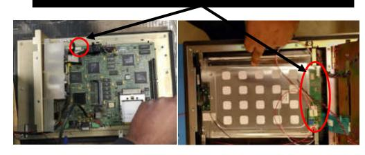
Unscrew the metal shields holding the CCFLs in the LCD Panel.
