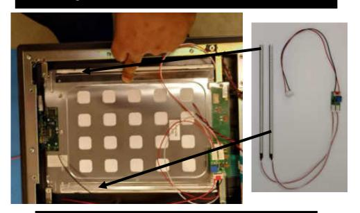
Mount the Inverter Board on to one of the screw holes that was mounting the old Inverter in place. Use the Nylon Screw and Nut the mount it.
