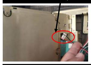
Connect our power adaptor cable to this connector on your controller board.
