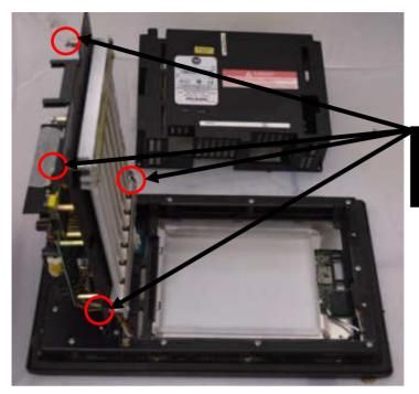
Loosen 4 screws and open hinge.
