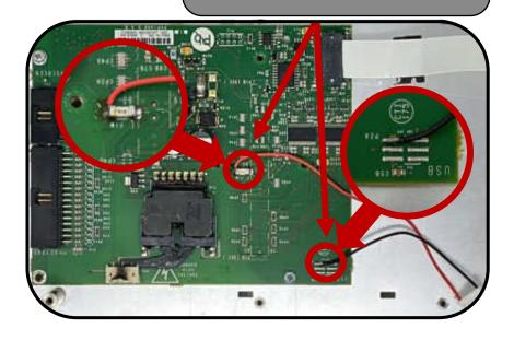
Locate the semi-circle notch and standoff in the metal work. Remove backing from double sided tape and stick down the inverter bd. Make sure that it is not covering the screw hole for the front bezel
