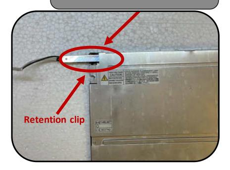
Carefully slide in new LED backlight into channel of LCD. Slide it all the way in until it stops
