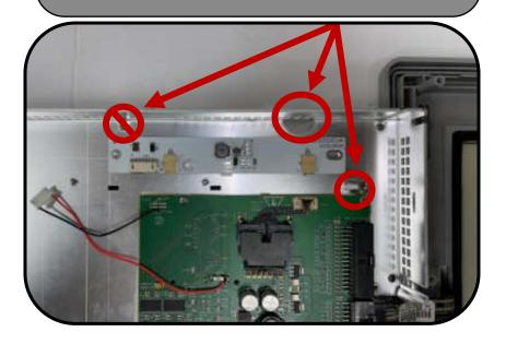
Plug the power cable and the LED strip into the inverter
