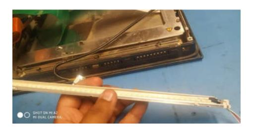
4.Attached the inverter cable into our inverter board and stick the inverter boards into safe no conductive places on the assembly.
