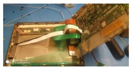
3.Unscrew the CCFL backlight out of the LCD Panel. Take the CCFL bulbs out of the housing. Take out the inverter board. Then stick the Monitech LEDS into the housing. Then mount the back light cover back in.
