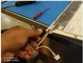
Step #6) Unplug the controller power 9 pin connector from CN1 of the NEC 121pw181 Inverter, Unscrew the inverter board off its mounting.
