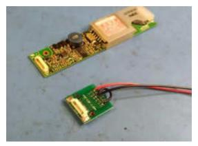
Step #8) Then slide in the LED backlight into the space where the old CCFL Bulb was. Use the zip tie provided to tie down access wires.
