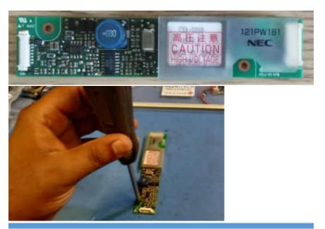
Step #7) Get the Monitech provided LED backlight replacement. MB121PW181 out of the bag. Connect the CN1 plug into out adaptor board. And mount the niverter boards with the double sided tape at the back or with the nylon screw set we provide.
