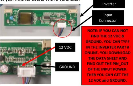
Step #5) Now that you have idenfitied the 12 VDC & GROUND you can take the wires out of its connector. Then connect the ground of the invertor input to our black coming out of our board. Then connect the 12 VDC of the invertor input to our red coming out of our board. Use the white dual clip connector to connect the wires together.
