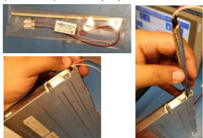
Step #4) Identify the the Ground and 12 VDC Wires on the input of your Inverter Board. With a Voltmeter.
