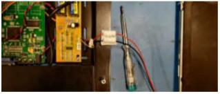
Step #6) Now mount our inverter board by using the double sided tape or using the the M3 Nylon hardware provided to you in the package. Use the zip ties to secure any loose wires.
