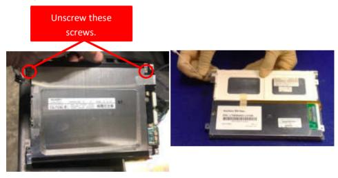
Remove the CCFL Bulb out of the backlight housing. Replace the bulb with the Monitech LED Backlight Strip. Remove the tapa cover to stick the LED Strip into the Backlight housing.
