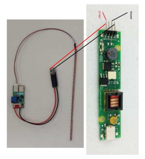
Located area on the back of LCD mounting plate and remove the release paper from the back of the inverter board. Stick inverter board down. Plug the LED backlights into the inverter board. It doesn't matter which connector you plug into.
