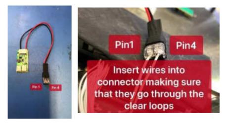
OR AND ALTERNATIVE SETUP IS TO US PIN 4 OF INVERTER SIDE CABLE (12 VDC) & PIN 2 OF INVERTER SIDE CABLE (GROUND). First Identify if they measure 12 VDC and Ground. The cut and strip the identified wires. Then attach 12 to red and G to the black wire of the connector going into out inverter.
