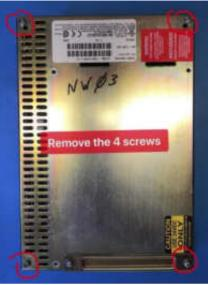
**Step 2**Remove circuit board
