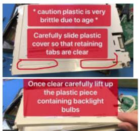
**Step 8**Remove old backlights and prepare housing for new LED bulbs.
