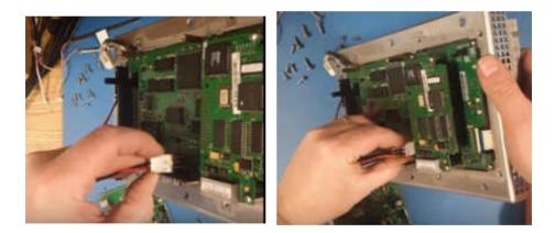
Place the power supply board back on and make sure the gold pin go through. Screw the board in place.
