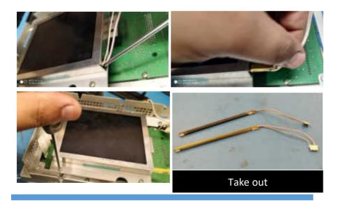
With a flat head screwdriver push down on tabs holding the lights in place. Now put in your Monitech LED backlights into the LCD panel.
