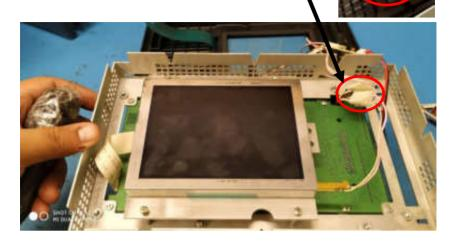
With a flat head screwdriver push down on tabs holding the lights in place. Then pull them out carefully. You might have to unscrew the LCD off its mounting to get the light fully out.
