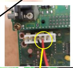
Connect LED power wire onto the terminal posts between main board and power supply.
