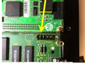
Insert red wire onto the pin marked 12.
