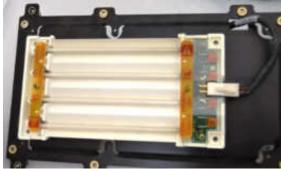
Open hinged access to original backlight by loosening two screws.
