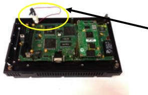
Remove the 4 pin squre plug from the assembly.
