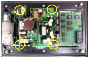
Remove power supply (4 screws).
