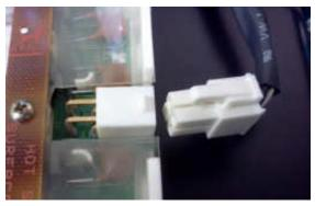
Remove the old backlight tray and disconnect cable. Keep screws handy.
