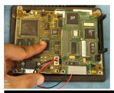
PLACE THE POWER SUPPLY BOARD BACK ONTO THE MAIN BOARD AND SCREW IT IN.
