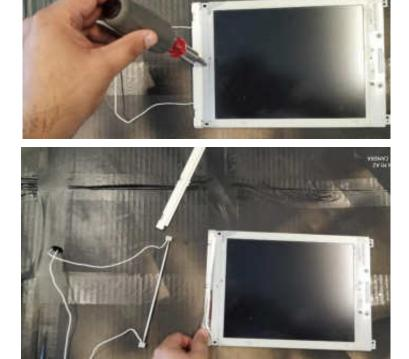
**Step #7)** Get your Monitech Backlight replacement. Put it in where the CCFL bulb used to be. Make sure the bulbs are directed towards the panel and is enclosed by the aluminum foil. We have provided you with a Aluminum tape to seal the foil, or if the foil is britle. Make sure the wire for the light go through the hole. Then put the cover of the backlight back on. Mount the LCD back into place.
