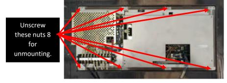
Step #3) Take off back cover the HMI by screwing the 4 screws.
