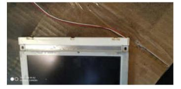
**Step #8)** Feed the boards and cables from our backlight though the hole. Then remove your orignal inverter by unscrewing the it and unplugging the blue inverter cable. Then plug the blue inverter cable into our board and mount the boards where the standoff of your oringal inverter used to be, or you can use the double sided tape at the back of our board to stick them where you please.
