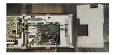
**Step #4)** Unplug CCFL connector from invertor & Unplug the LVDS cable from the LCD Panel. Then unscrew the 4 screws holding the LCD mounting plate in place.
