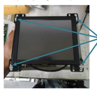
With the screwdriver fasten the 4 screws to attach the New Monitech Monitor on these 4 holes.
