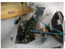
Unplug the Yoke and the Unscrew the Yoke Ground from the Frame.
