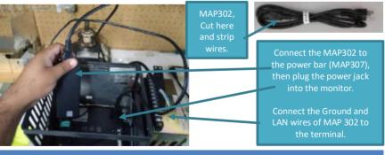
Option 2) Cut the jack part of the MAP307 (Power supply) and strip the 2 wires. Solder or use butt connectors to connect the red wire to controller to red wire of jack. Solder or use butt connectors to connect the black wire to controller to black wire of jack. Then plug the jack into the monitor.
