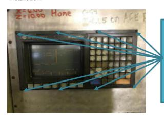
To see the CRT and controller you must remove the back panel by unscrewing the screws hold it.
