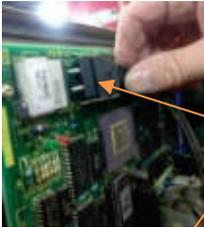
Reconnect all the connectors removed at the beginning of the Installation
