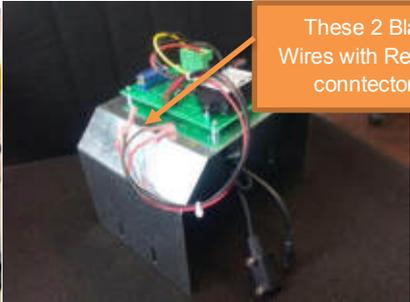
Do this same process for the 24 VDC Wires and Cut them for original connector, strip them and crimp them to our 2 red wires with red butt connectors.
