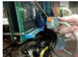
**Step #11)** Plug the BLUE Video connector into the blue socket as shown below. Plug VGA from the Adaptor to our monitor, and the power jack.
