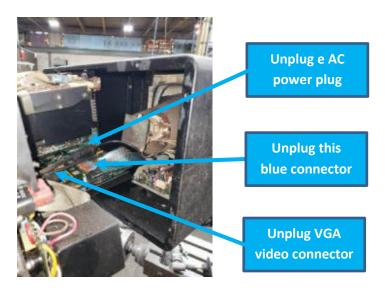
**Step #7)** Unscrew the screws holding the white bezel inside the console. Then take out the CRT, then unscrew the Black Bezel out of the console. Keep the nuts removed for reinstallation.
