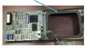
Step 2) Put the brackets on the monitor with the original screws from the CRT. Take off the hardware that is on our monitors mounting hears first. Use the side screws of the bracket to side the metal down bracket down.
