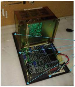
Take the HMI off the machine by unscrewing each screws that board the interface.
