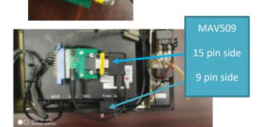
Step 5) Mount the board onto the monitor with the use of the 2 standoffs in the MH948. Then stick them on the monitor.
