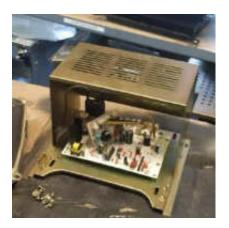
Step 9) Take the Monitech monitor out of the box and mount it on to the brackets taken off the CRT Frame as shown using the hardware on the Monitor. Mount it back into the HMI with the 4 screw that held the old CRT Frame on the HMI. Or use the existing screws from the CRT frame to mount our monitor.
