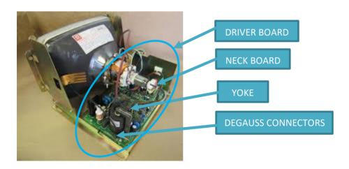
Step 5) Unscrew 4 screws holding the CRT in place. Remove CRT from the frame. KEEP THE SCREW FOR INSTALLATION.
