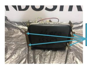
Unscrew these nuts holding the CRT frame in the HMI
