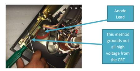
Step 4) Remove the Anode Lead, Yoke, Neck Board and Degauss connector to remove the driver board from the CRT frame.
