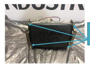
Unscrew these screws holding the CRT in place.
