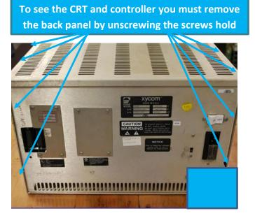
**Step #4)** This is what you got. Unplug the power & video cable off the driver board & CRT Housing.
