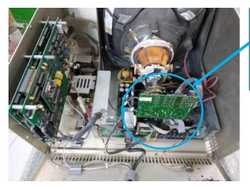
REMOVE THE DRIVER BOARD FROM THE ASSEMBLY.
