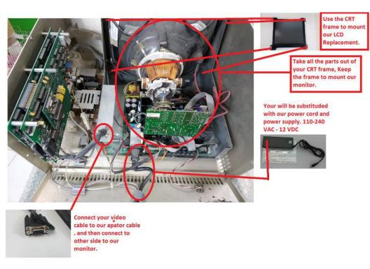
**Step #9)** Before Mounting the HMI back into the machine. Turn On power and Main Power to test the Monitor. If Video is on use the User Guide to Adjust the Screen. Then mount the HMI back into the machine. Then do Steps 1-3 in reverse.
