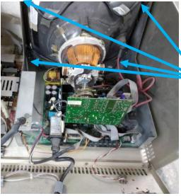
Unscrew these 4 screws to remove the CRT from the Housing
