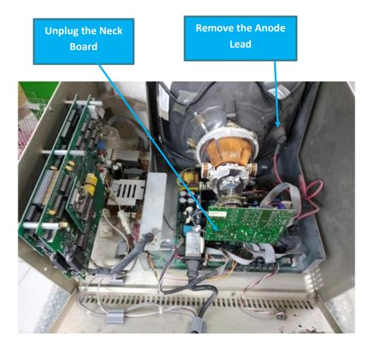
**Step #6)** Take the CRT Housing out of the HMI Frame. Make sure to keep all the screws for reinstallation.
