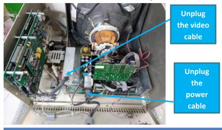
**Step #5)** Remove the Anode lead from the CRT, with a flat head screwdriver. Remove the neck board from the CRT.
