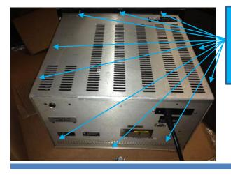
Unscrew the nuts from these studs to take the HMI out of the machine
