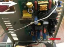
**Step #5)** Take Anode Lead off the CRT with pliers. Unplug Degauss Connectors off the CRT. Unplug the Yoke connectors from the CRT off the Driver Board.
