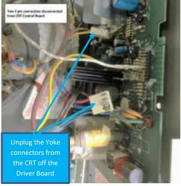
**Step #6)** Remove the Driver Board out of the HMI. Remove the CRT out of the HMI by unscrewing the 4 screws holding in place. Keep the 4 screws for installing your Monitech Monitor.
