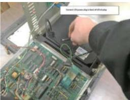
**Step #8)** Connect the MAV097-A into your controller Video & Power Cable.
