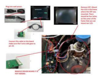
**Step #9)** Before Mounting the HMI back into the machine. Turn On power and Main Power to test the Monitor. If Video is on use the User Guide to Adjust the Screen. Then plug the controller power connector back into the power supply. Mount the HMI back into the machine. Then do Steps 1-3 in
