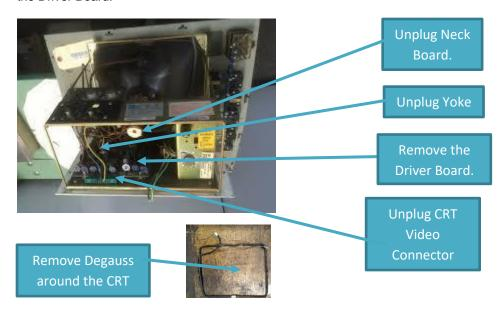
**Step #6)** Unscrew the 4 screws holding the CRT monitor on the frame. Take the CRT out of the frame. Keep the 4 screws just removed for install your Monitech Monitor. Now you are left with the CRT frame.
