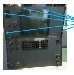
Take the Front Cover of the HMI by unscrewing each of the following screws. Keep the screws for re- installation.
