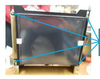
Now mount your Monitech monitor onto the old CRT frame, using the screws removed in Step #6 **Step #8)** Use MAP315 + MAP307 to adaptor to the AC power. Then plug in the jack into our monitor. Plug in the BNC connector from your controller into the BNC board on the CRT FRAME. Connect MAV077 into the green connector. Connect the VGA side of MAV077 into our monitor.
