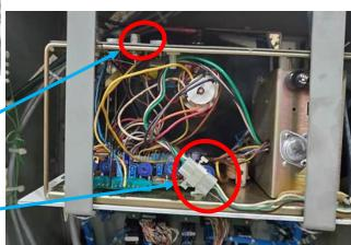
**Step #3)** Remove the CRT Frame with all the electronics from HMI by unscrews the screws holding it in place. Keep these screws for reinstallation.
