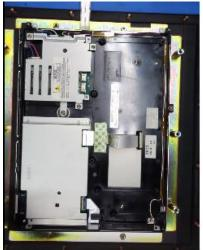
**Step #7)** Remove the LCD from the HMI, by unscrewing the 4 screws that Is mounting the LCD.
