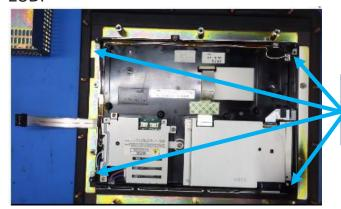
Unscrew these screws to remove the LCD Panel
