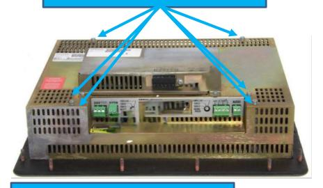
Remove the board, by unscrewing the board.
