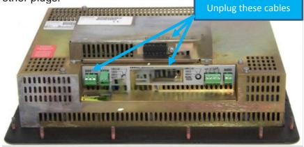
**Step #3)** Remove the HMI out of the machine by Unscrewing the mounting nuts around the HMI. Keep nuts
