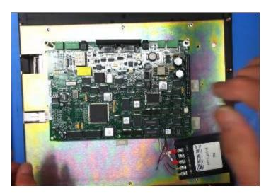
**Step #13)** Mount the back cover back with the screws and then power up the HMI with 24 VDC. Then mount your HMI back in your machine.
