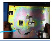
**Step #12**) Mount the board back onto the middle metal. Then connect your touch screen cable back on the board. Mount the power supply back on the middle metal.
