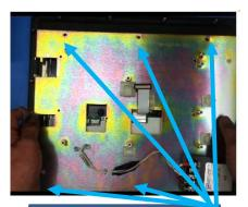
Unscrew surrounding screws to remove the middle metal off
