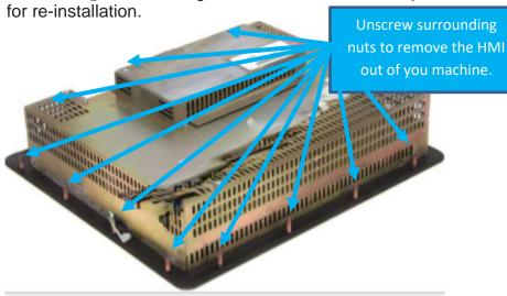
**Step #4)** Remove the back metal & the board from the HMI by unscrewing the following screws. Keep screws from re-installation.
