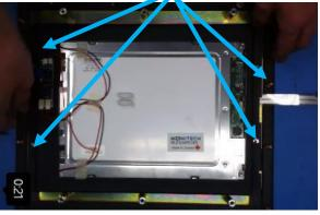
**Step #9)** Get the board removed in Step # 4. Get the LVDS Cable from our box. Plug it into the LCD and the Board.
