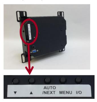
Now press **AUTO** on the 5-button menu found on the back of the LCD. After a few seconds, the screen will center the image and automatically adjust the image size, color, brightness and contrast.
