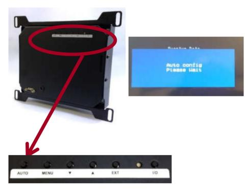
Now press **AUTO** on the 5-button menu found on the back of the LCD. After a few seconds, the screen will center the image and automatically adjust the image size, color, brightness and contrast.
