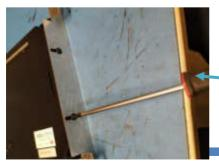
Place the brackets where the slots are. Use the screws previously taken off to fasten the brackets.
