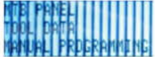
In the 3-button menu, select WIDTH and adjust values until the lines disappear. When you have done all you can do with this setting, select PHASE to fine-tune it.
