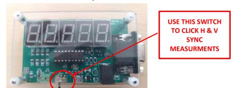
STEP #4) IF YOU ARE NOT GETTING ANY READINGS, OR ODD NUMBER READINGS. YOUR VIDEO CARD IN YOU CONTROLLER IS NOT SUPPLING THE PULSES TO THE ADAPTOR CABLE. OR OUR CABLE HAS THE WRONG PIN OUT.
