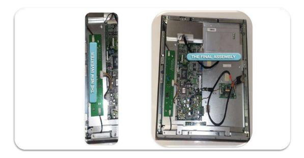
• After you install the front panel that has the new inverter to the main unit, and before you power up the unit, make sure everything is connected properly and safely to power up.
