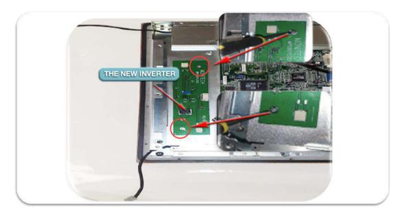
• Insert the LED strips cable to the connectors of the inverter and then insert the power harness to the power connector of the inverter.
