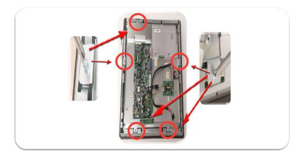
• Remove the LCD panel by unscrewing the 4 screws, then pull up the LCD panel from the metal frame.
