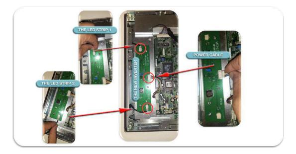
• The new inverter after it has been installed.
