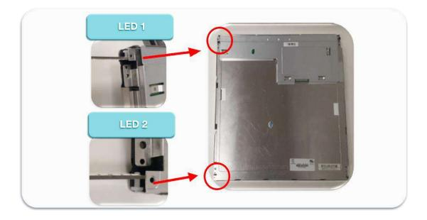
• Continue sliding the LEDs all the way until they fit completely as shown in the picture below.
