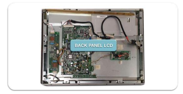
Disconnect the LVDS connector from LCD panel, then disconnect the touchscreen connector.
