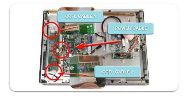
• Remove the old inverter by unscrewing the 2 screws as shown.
