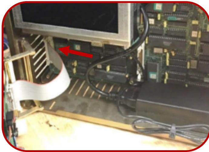
Connect the video cable back to the proper connector and attach the GND wire to C13.
