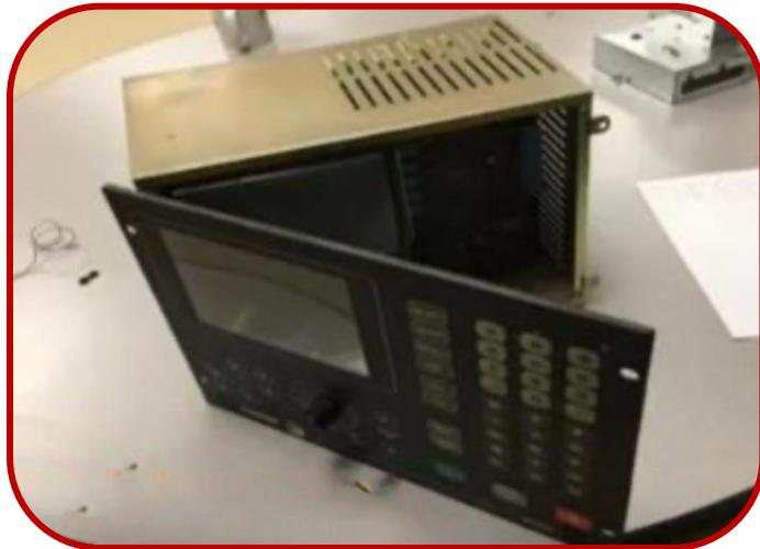
Remove the two nuts holding the hinge onto the front panel. Remove the PCB and selection switch. Unplug the user control cable from inside the controller.
