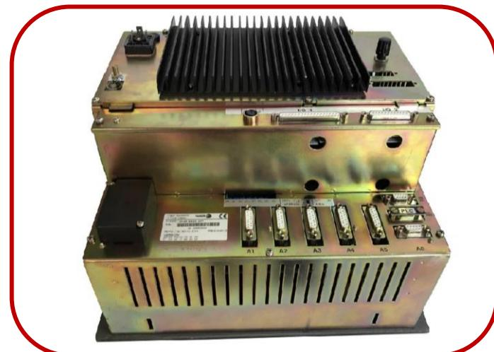
Remove thumb screws to get access to the I/O Card and remove it.
