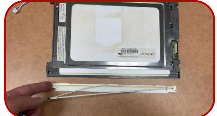
Step 6 - Route backlight wires through holes and plug into U3 and U4 of MB104S840C inverter.
