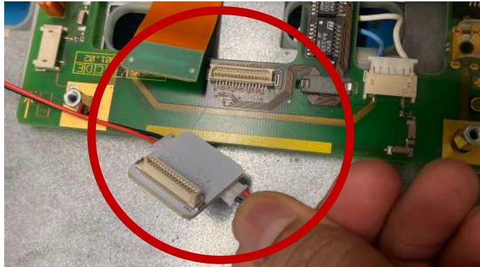
Step 3 - Carefully plug the video cable into MPCB044.
