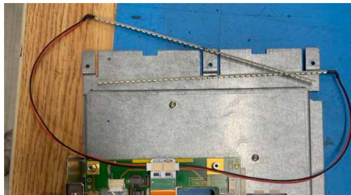
Step 2 - Orient MPCB044 in the right direction and carefully plug it into the connector.
