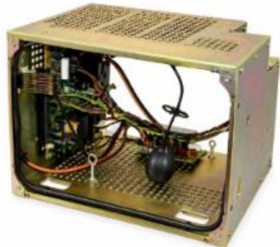
Remove CRT-frame fasteners
